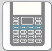
25-key keypad with 2 function keys and 28-key keypad with 4 function keys to fulfill user demands in dedicated function assignments.
