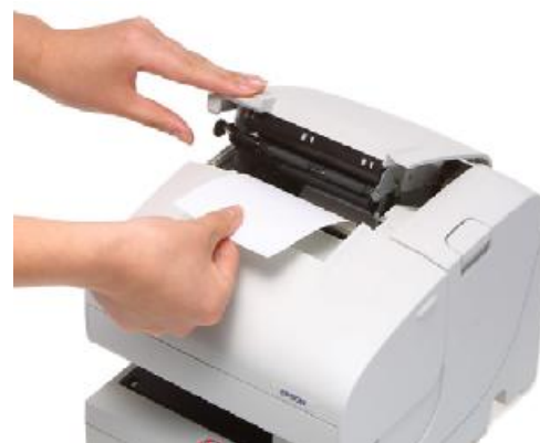
Open cover, drop in paper roll, close cover! That easy is the paper load for all TM-J
